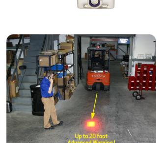
The Safe Spot has two LED lights and lenses to ensure a visible red spot on the floor and an excellent heatsink design to ensure long LED life.
